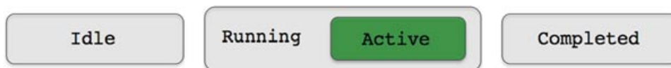
Figure 9. Behavior states: A behavior may be in one of these four states at any given iteration of the helm Iterate() loop. The state is determined by examination of MOOS variables stored locally in the helm's information buffer.
