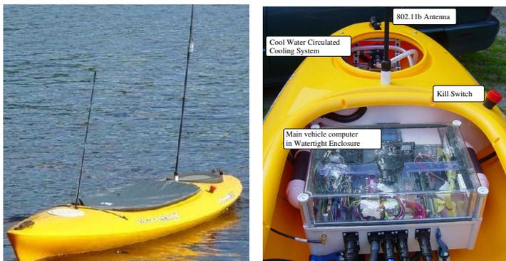
Fig. 6. The kayak-based autonomous surface craft.
