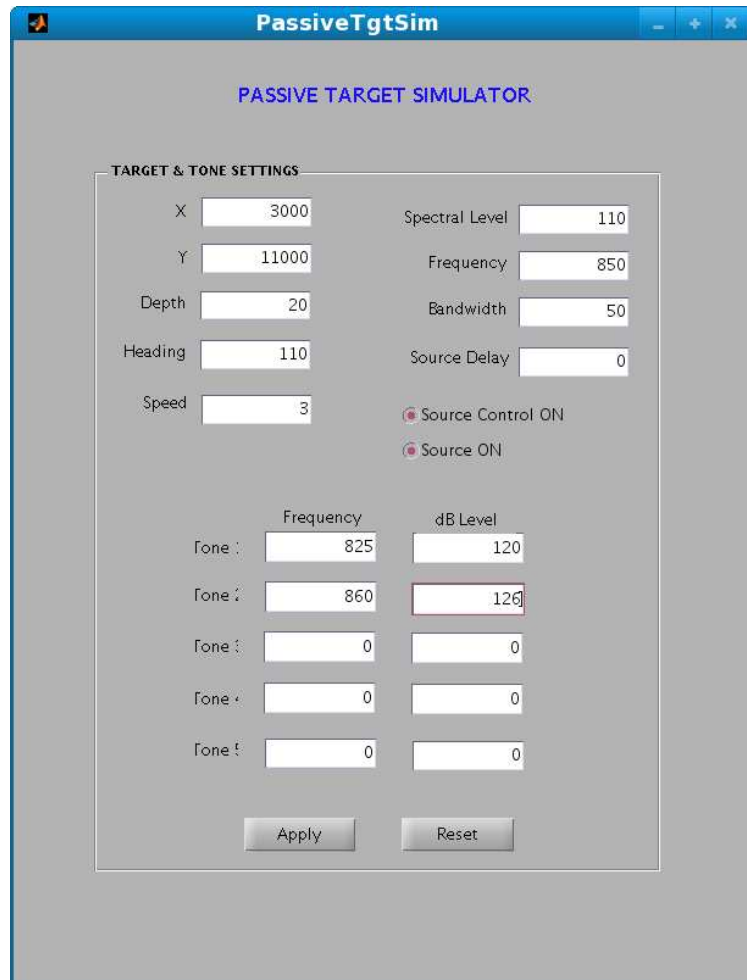
Figure 27: PassiveTgtSim.m: GUI for activating acoustic sources to be dynamically simulated by pMultiTargetSim.
