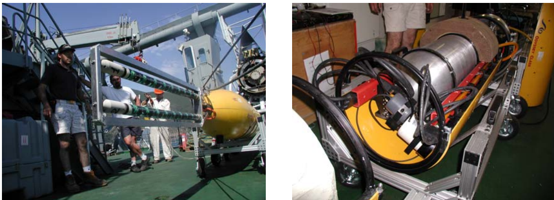
Figure 1 GOATS'2002 Odyssey III acoustic payload. (a) Twin line array mounted in nose of the AUV. (b) Pressure vessel with 16 channel DSP-based acquisition system, and Edgetech sub-bottom profiler source configured for insonifying the seabed at 30 degrees grazing angle.
